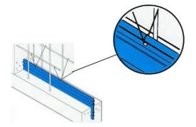
**MasterSeal 940** ECJ & EEJ profiles when used on ground slab blinding concrete where a permanent, firm and stable support is given usually require no fixing. The profile is simply laid centrally over the line of the joint to be formed. Fixing to vertical shuttering is simplified by nailing with double headed nails through the outer reinforced flange to provide a firm fixing as shown below.
